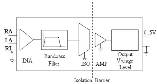
Fig. 2. Block of ECG signal conditioning.
