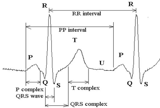
Fig. 1. The patterns of real ECG signal are waves, complexes and intervals defined in this figure.
