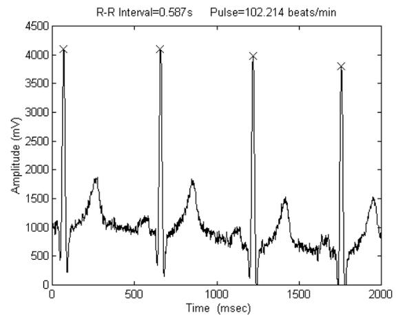
Fig. 5. The detection of R points and calculus of the cardiac frequency.
