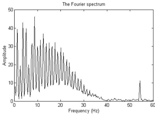
Fig. 9. A graphical representation of the Fourier spectrum for an ECG unfiltered signal.
