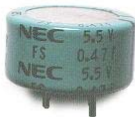
Figura 5.17: Condensator “double layer”
